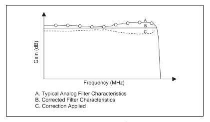
Figure 2-13. Analog Filter Correction
